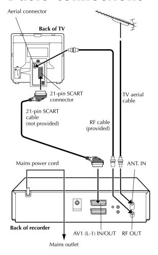
Make AV connection if your TV has a 21-pin AV input connector (SCART) in order to reduce the possibility of interference. With AV connection, you can enjoy stereo playback of video tapes if you are using a stereo TV.
